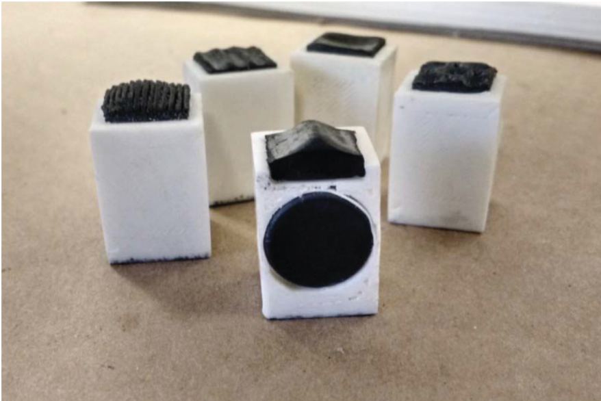
Fig. 2. The physical icons used in the Tangible Desktop (see Figure 1). Each icon has an RFID tag embedded inside and a tactilely distinct rubber crown.
