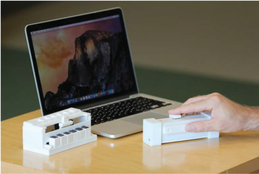
Fig. 1. A picture of the Tangible Desktop in its standard arrangement. The Tangible Taskbar sits to the left of the laptop while a user engages with the thumb of the Tangible Scrollbar.
